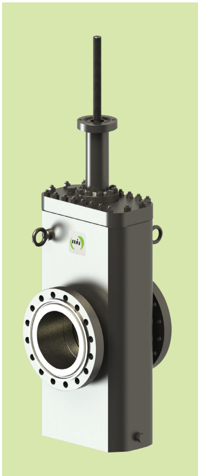
MV7-F-SS Subsea Forged Gate Valve 10" CL.300 RTJ Forged Body LTCs with SS weld overlay on all wetted parts, Duplex trim, TCC hardfacing, lipseals High pressure gas testing, 35m depth, Malaysia
