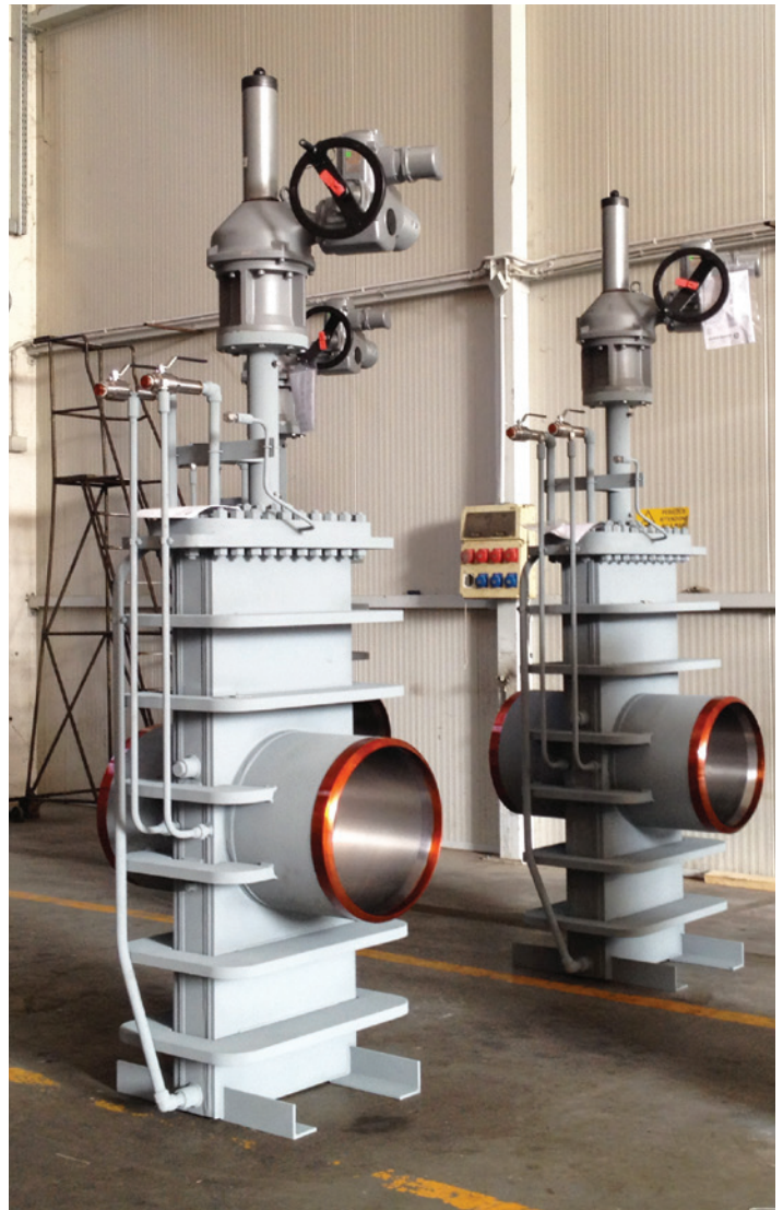
MV7-P Through-Conduit Fabricated Gate Valve 20" CL. 400 BW Body and Gate A516 Gr.70, Stem 17-4PH Underground installation, Europe
