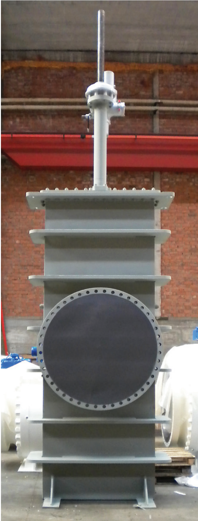
MV7-P Through-Conduit Fabricated Gate Valve 20" CL. 400 BW Body and Gate A516 Gr.70, Stem 17-4PH Underground installation, Europe
